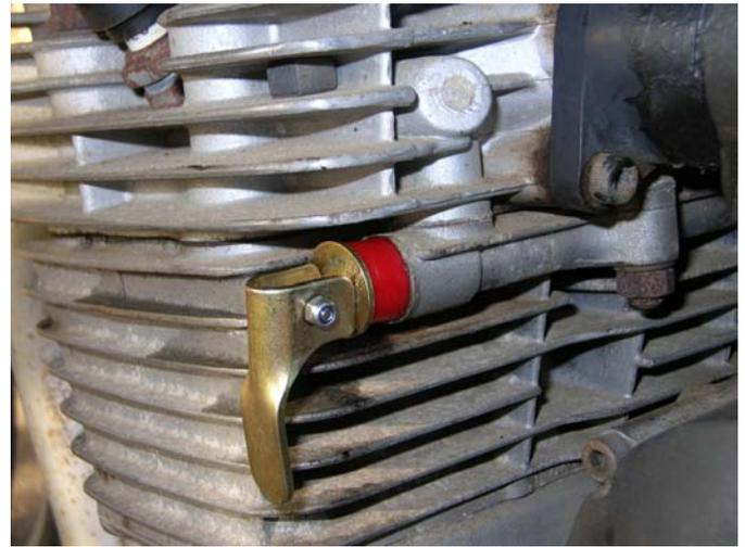
Flip down the trunion (locking) lever to expand the rubber seals and lock the tool into the cylinder. If the tool is not REALLY tight in the YICS passage, remove the tool and tighten the adjusting nut at the end of the tool slightly, put the tool back in and try again. The tool, when locked, should not be movable within nor removable from the passage.
