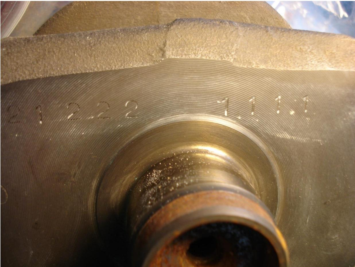
On the left side of the crankshaft, on the large flat counterweight, you'll find two sets of stamped numbers:
