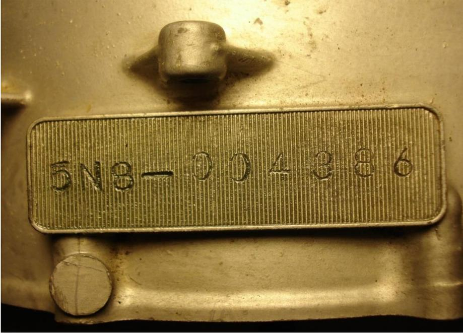
On the upper engine case, just behind or just beside the clutch cover on the right side of the engine, you will find a small, flat “ribbed” (to prevent re-stamping) machined pad that faces up (towards the sky).
