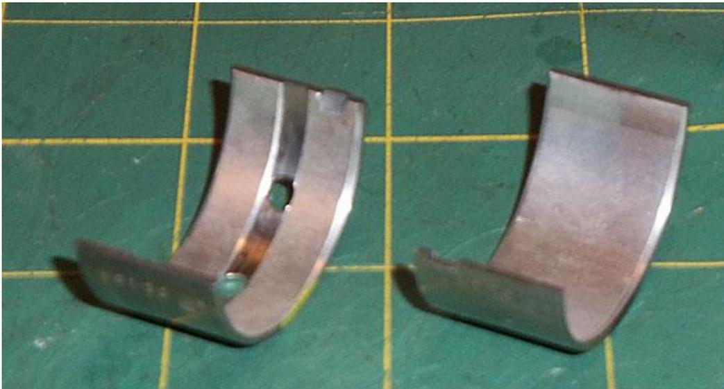
2) there are two different types of crankshaft main journal bearings: those **with** and **without** oil passage holes:
