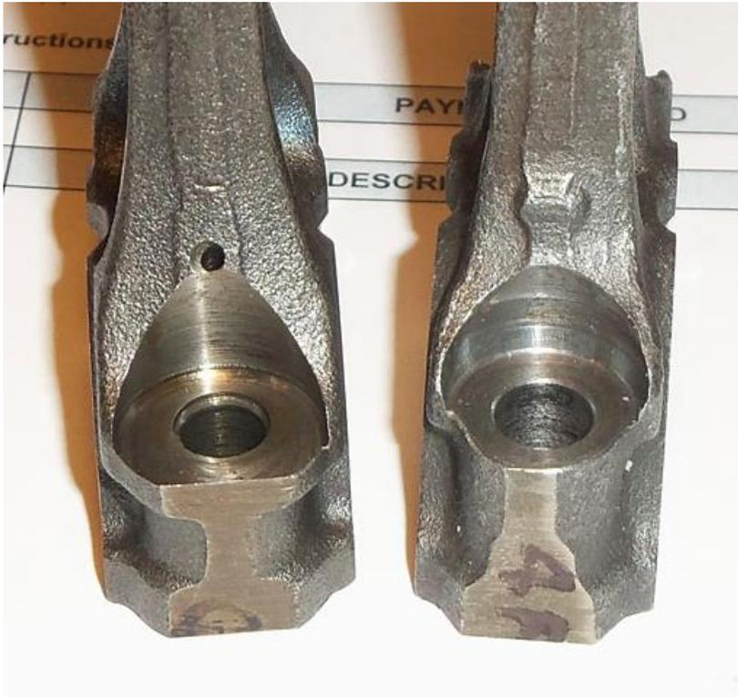
The oil spray passage hole allows pressurized oil to be sprayed onto the cylinder walls, aiding lubrication of that area.
