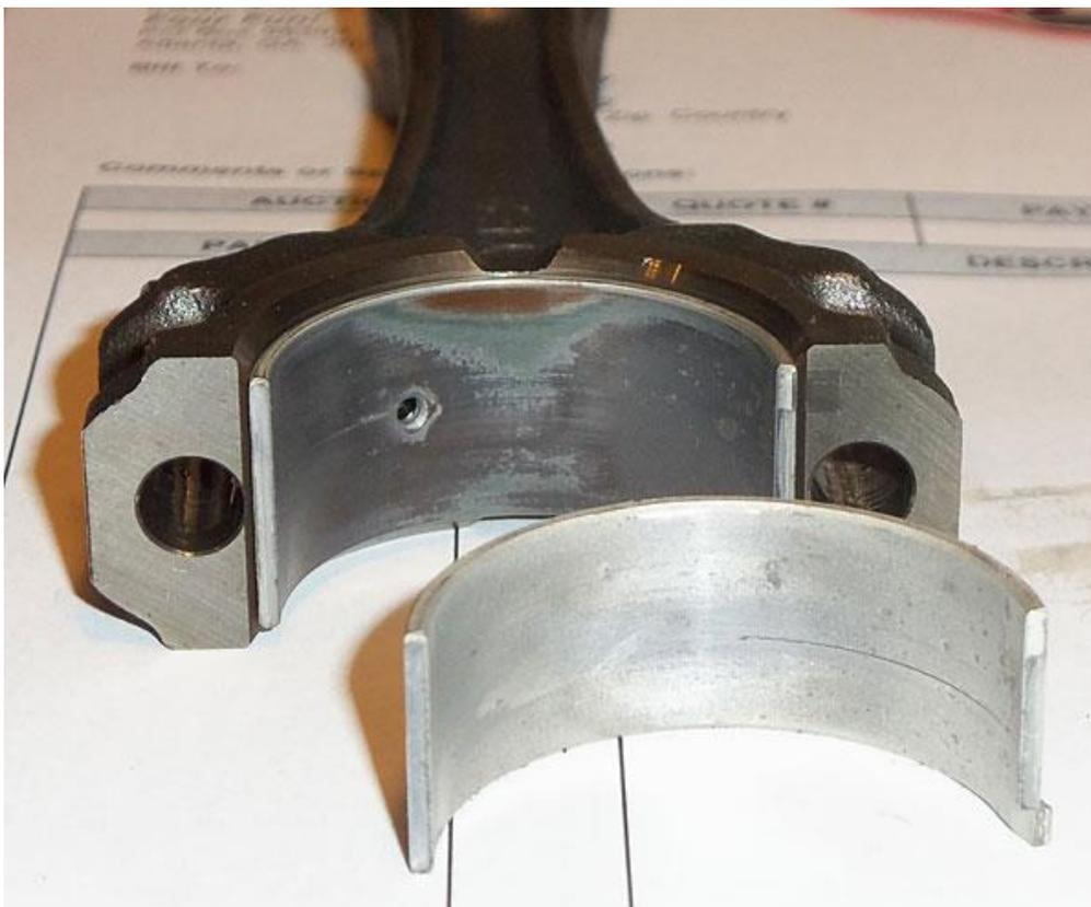
Obviously, rods which have the oil spray hole **MUST** use the bearing shell that has the spray hole passage hole in it:
