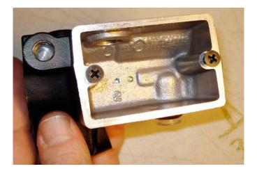
This is the first type we're concerned with. In the left picture, note the insert plate with the three curved slots. (Some had a single horizontal slot.) That insert is sealed in place with an o-ring, which is shown below. On the right, see how nothing extends into the cavity itself. (If you've noticed that it looks suspiciously free of grime and gunk, remember that cleanliness (and bead blasting) are next to godliness.)
