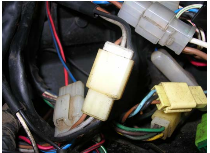
Tach input wires - ours is electronic, and does not require its own cable.
