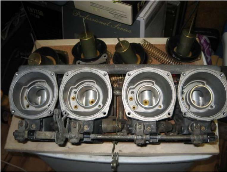
The springs and diaphragm/pistons are out
