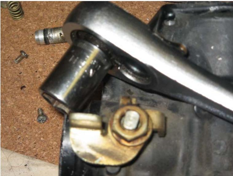
For the inner two bodies, the nut holding the shaft in wants a 12mm wrench/socket
