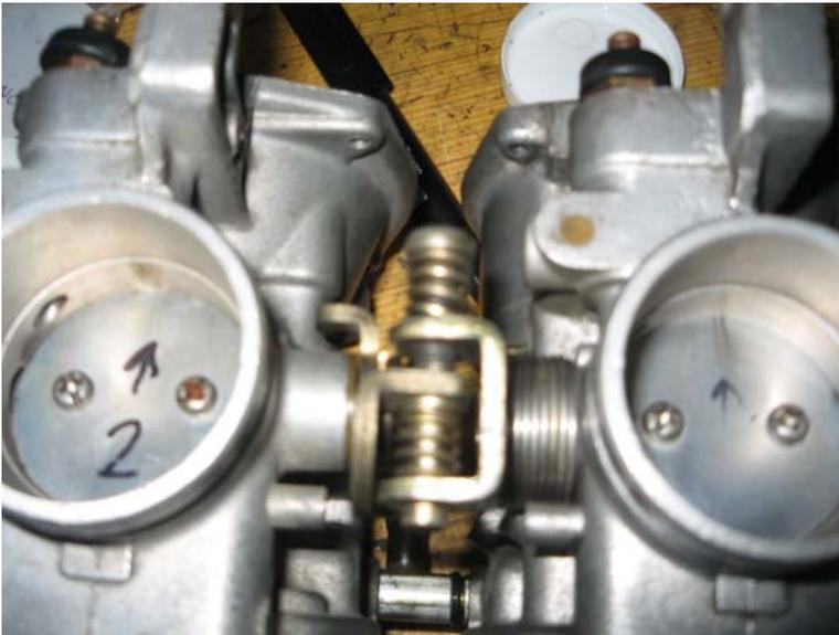
Slide the tab from the neighboring throttle shaft between the adjusting screw and the stud
