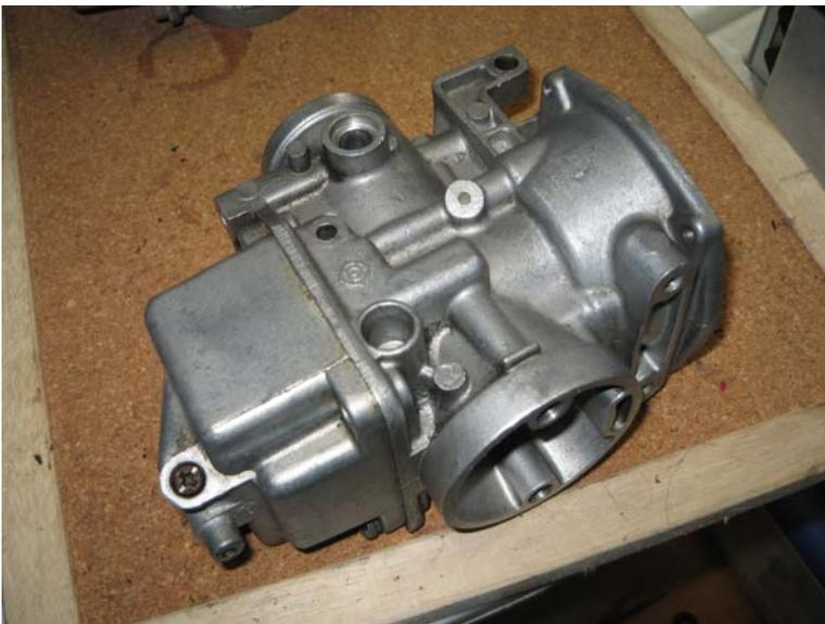
Switching back to my (somewhat cleaned up) working set now. Note that I've reinstalled the float bowl; it's been suggested to keep it bolted on to protect the float pillars from damage.
