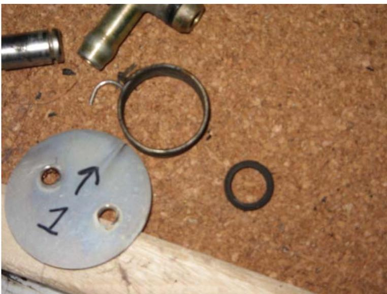
The butterfly, throttle shaft spring, and outer seal
