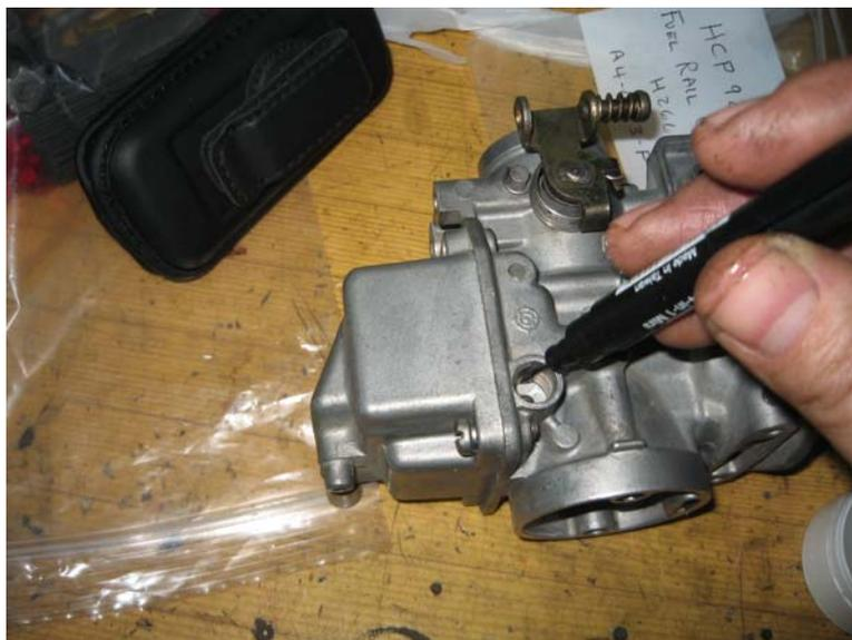
A thin coat in the hole where the tube goes...
