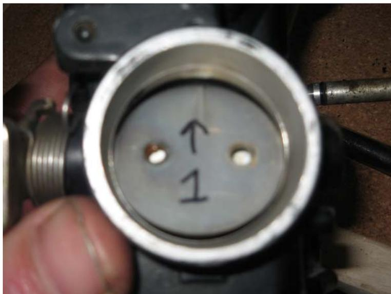
Remove the two screws holding the butterfly to the shaft
