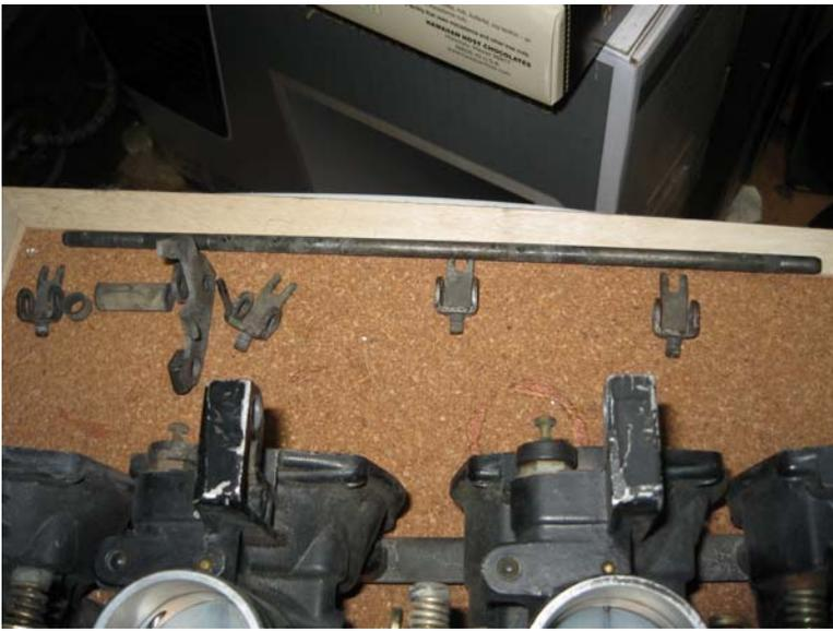
...and the starter plunger shaft is off. It's not necessary to completely take the set screw out; the better to keep track of.
