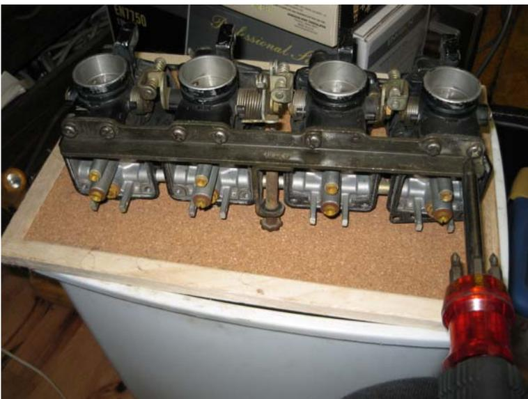
Remove the mounting screws from the bottom bracket
