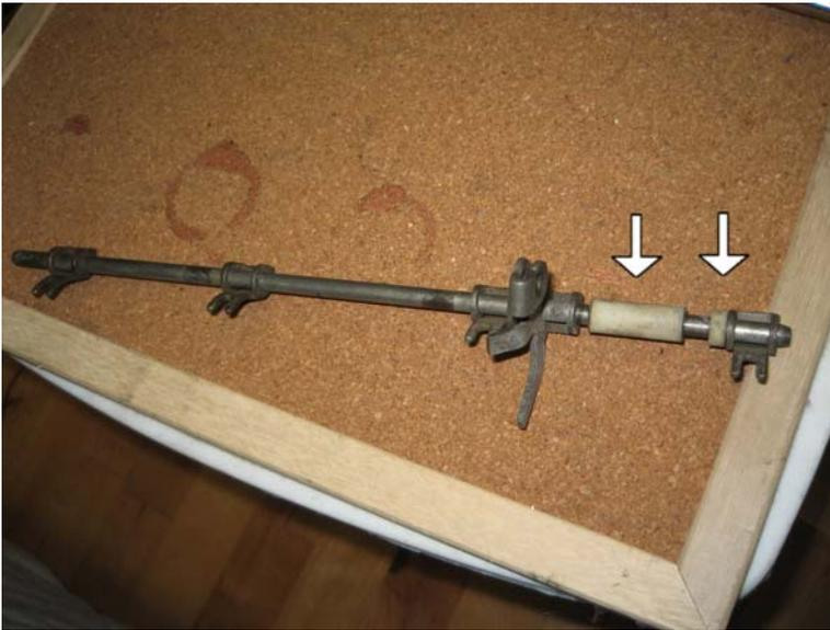
Here's a shot of the shaft removed, #4 side on the right. Again, note the spacers.
