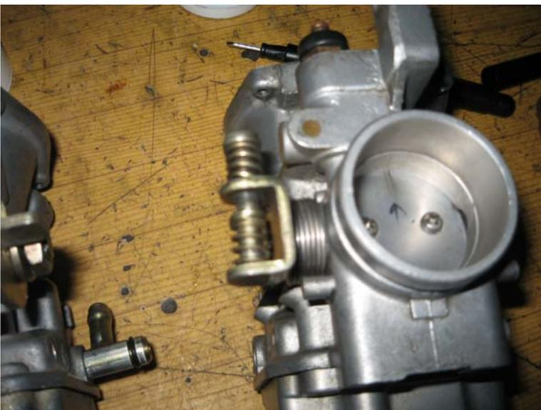
Stick the stud and spring back in the hole and put some tension on it
