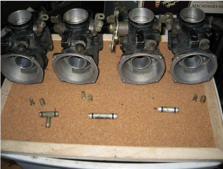
The fuel rail tubes (with o-rings) and the little studs/springs from the bottom part of the sync screws. Don't lose them!
