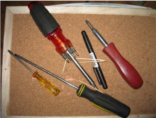
A set of good-fitting screwdrivers. Stripping the screw heads is a Bad Thing™.
