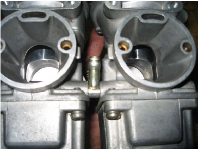
Press the other side of the fuel rail tube into the other hole
