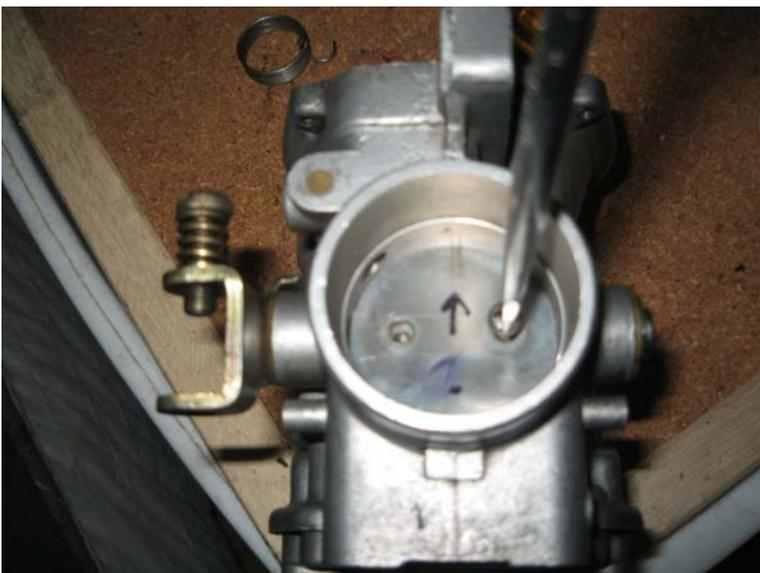
Reinstall the screws (remember that Loctite?)
