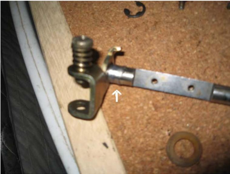
We put a thin layer of grease on the shaft...
