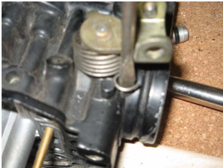
Unhook the spring from the throttle shaft
