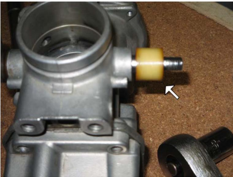
When you get to the #3 carb, don't forget that instead of a shim on the one side, it uses a largish spacer
