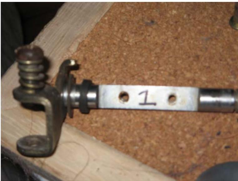
Probably a good idea to mark the throttle shaft, too. Note the other shim and seal still on the shaft
