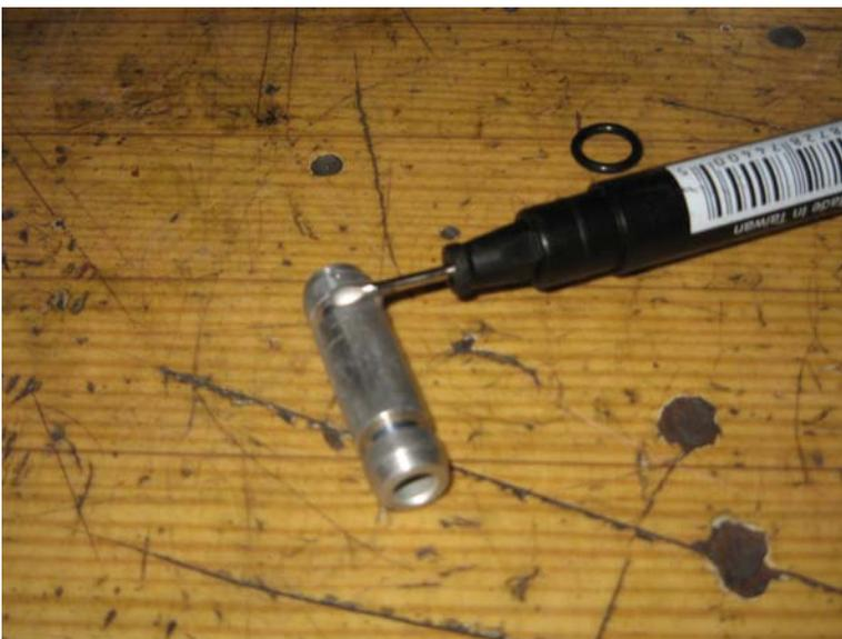
A light coat of silicone grease in the groove that the o-ring goes into
