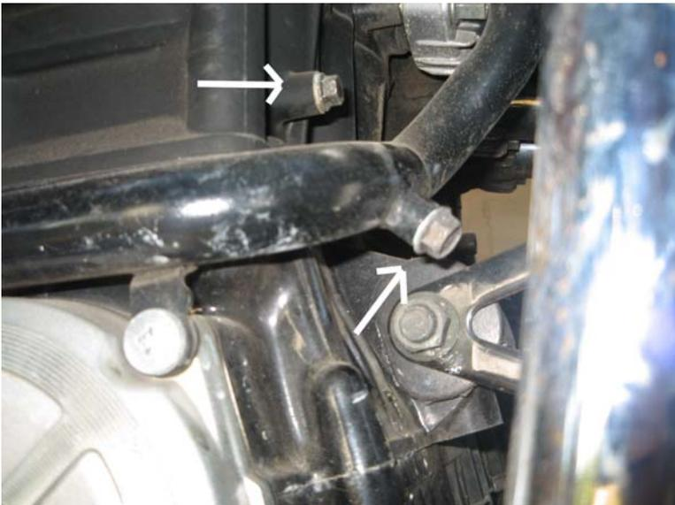
Right-side cylinder drain bolt (8mm) and radiator pipe drain bolt (10mm)
