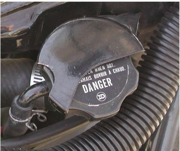
If you have the guard that goes over the radiator cap, remove it. It's held on by a 10mm bolt (or so I'm told... I don't have one).
