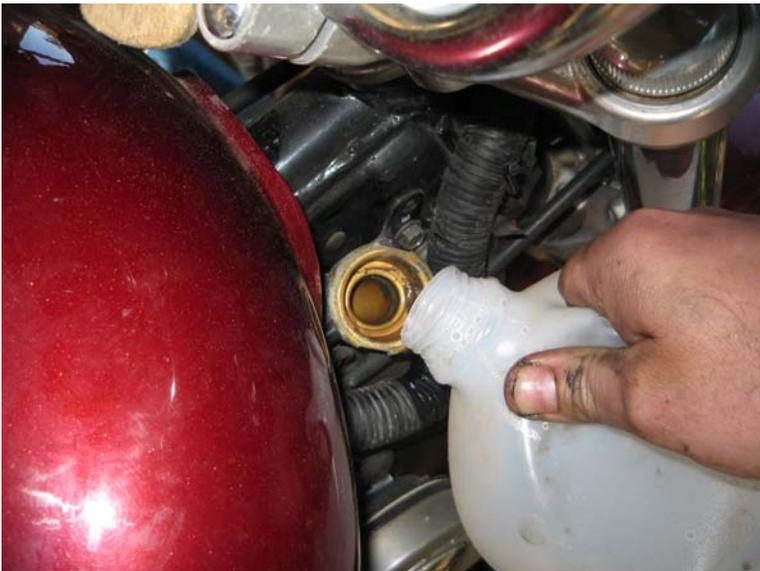
Pour the stuff in until you're up to the neck, then go around and pull the drain bolts one by one again. You'll probably want to do this procedure a total of two or three times, making sure you've drained all the water after each fillup.
