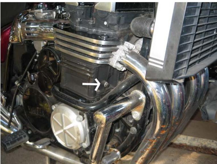
Right-side cylinder drain bolt
