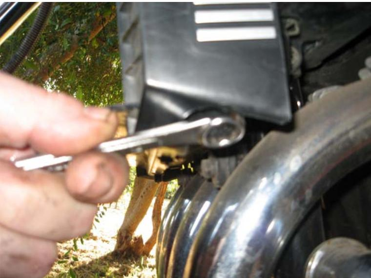
Next, grab your 12mm and loosen the radiator drain bolt.
