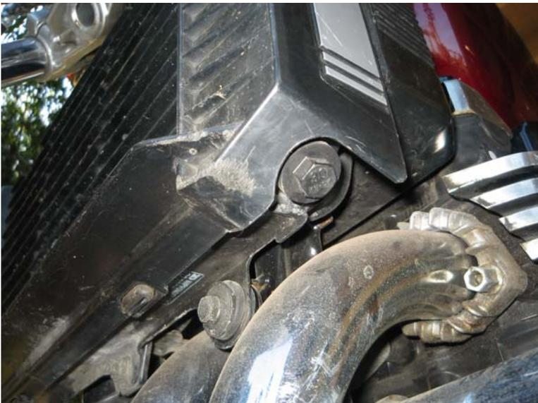
A better view of the radiator drain bolt. Funny that the bolt here is on the left side of the radiator, when the parts diagram shows it on the right side...
