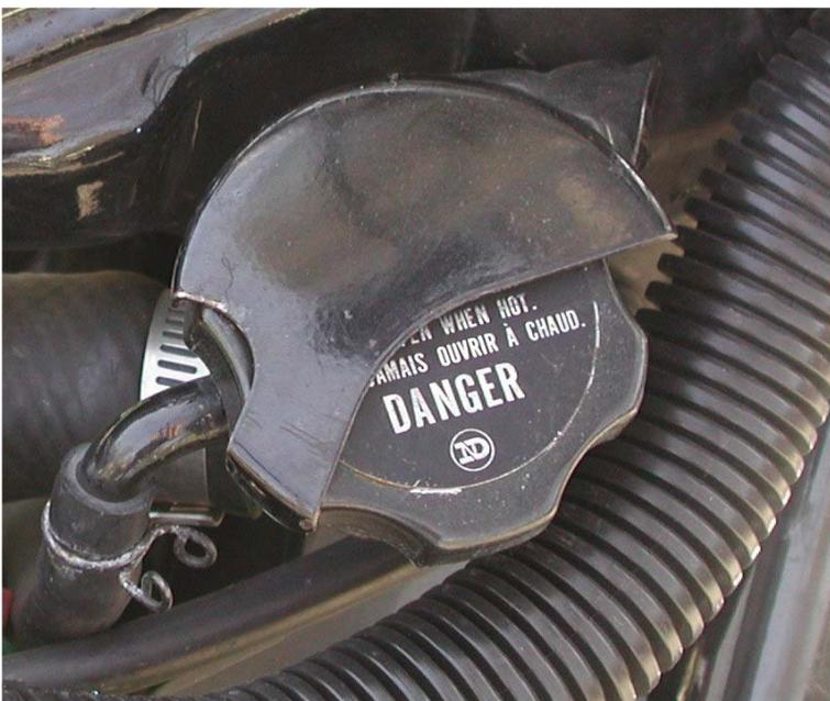
If you have the guard that goes over the radiator cap, remove it. It's held on by a 10mm bolt (or so I'm told... I don't have one).
