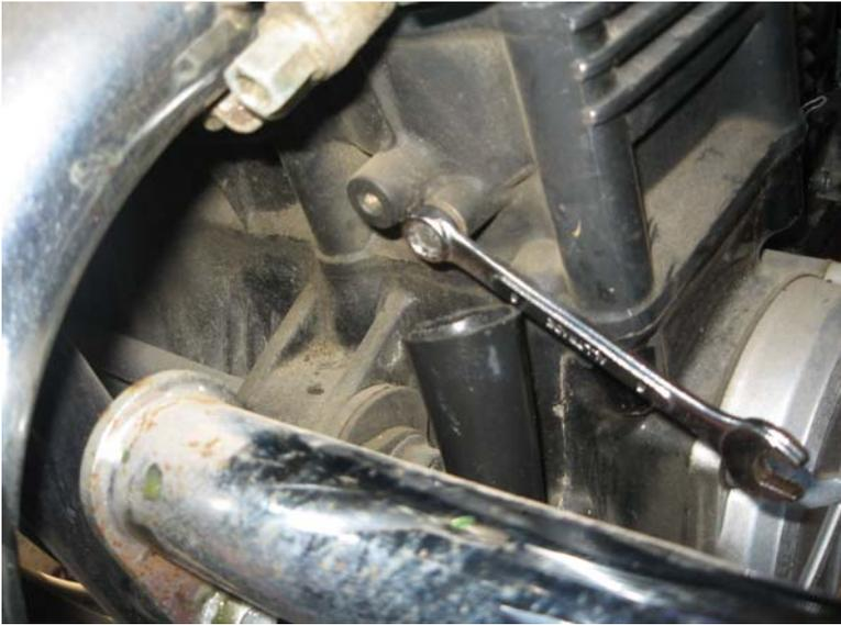
Once the radiator is done, next up is the left cylinder drain bolt (8mm). The funnel likely won't fit in here, so if you have that flexible tube like I mentioned earlier, it will come in very handy.
