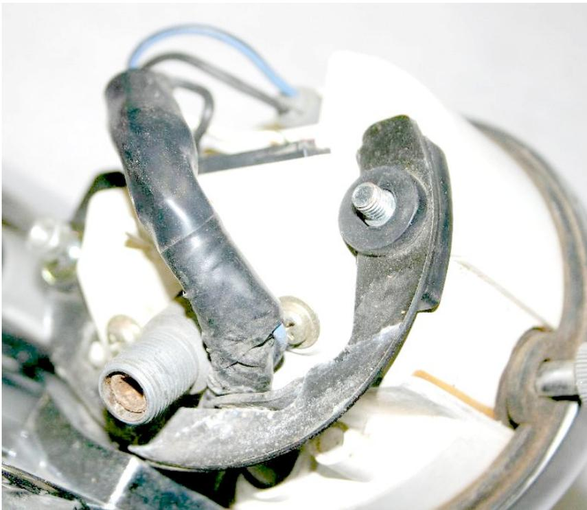
Once the cover's off, you can remove the nuts and washers for the mounting bracket, then the bracket itself.
