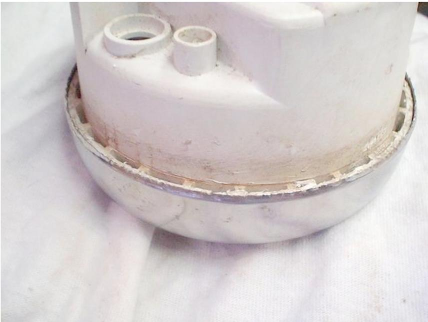
Keep working your way around the edge of the bezel until you have loosened it up enough to slide out the gauge body. Set the body aside.
