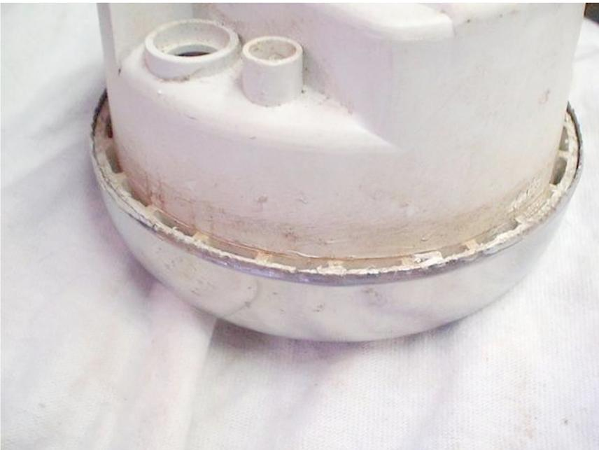
Place the gauge body back into the bezel. Take a large blade screwdriver, or a wide punch, and start folding the bent-up portion of the bezel back down over the edge of the body. Work in a star pattern to ensure that the body doesn't sit off-kilter in the bezel.
