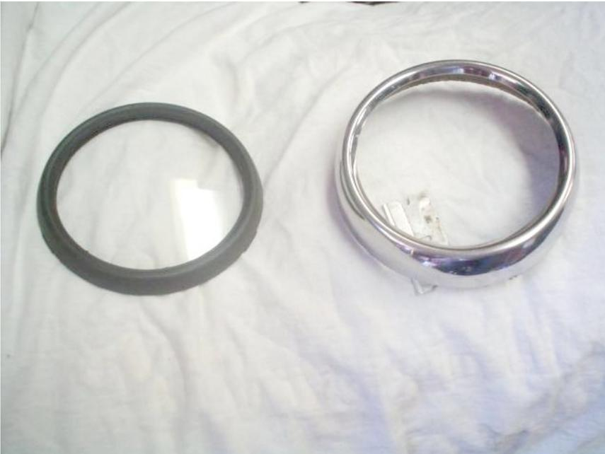
In our example, we've borrowed an intact glass piece from a junked gauge; this is notable because the original glass pieces are slightly convex (bulging outward). Unless you can source these (new or used), your replacement glass piece will likely be flat.
