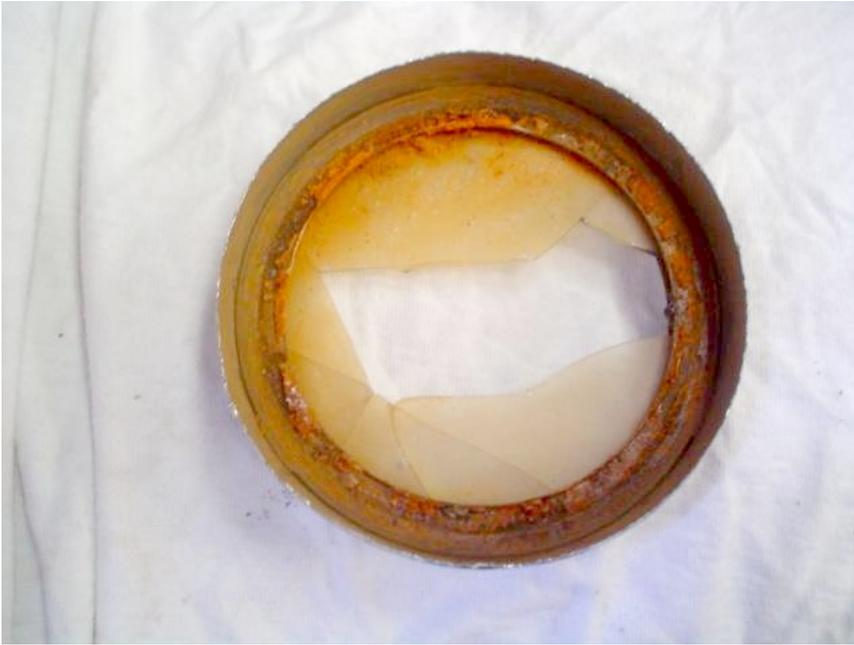
Carefully press the glass/rubber/metal ring out from inside by pushing from the front of the glass.
