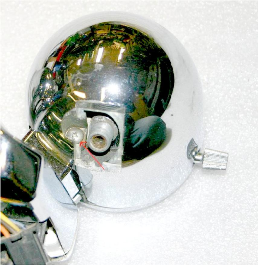
The red arrow here points out the retaining screw for the outer cover.
