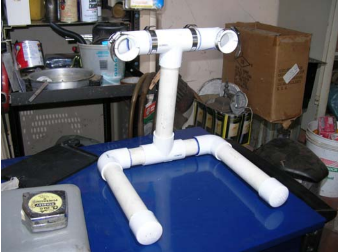
A carb stand of some sort, to hold the carb rack level and upright. This wonder of PVC was inspired by a user from the Kawasaki Concours forum.
