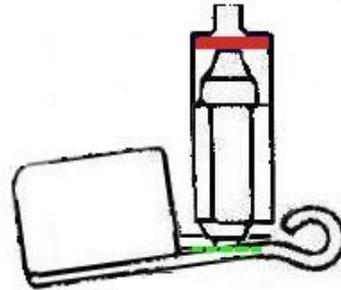
With the carbs sitting upright; if you bend the tang arm (in green) **down**, away from the carb body, that will increase the gap (shown in red, above right). More fuel will enter the bowl, the floats will have to rise farther in order to lift the needle and plug the hole in the valve seat, and the fuel level sits closer to the top of the bowl. Thus, the **fuel level measurement decreases**.
