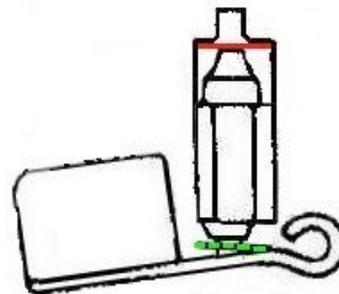
Conversely, if you bend the tang arm (in green) **up**, toward the carb body, that will decrease the gap (shown in red, above right). The floats won't have to rise as far to lift the needle and plug the hole in the valve seat. Since less fuel enters the bowl, the fuel level sits further away from the top of the bowl, and thus the **fuel level measurement increases**.
