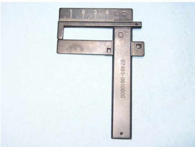
A float height gauge ( HCP4 , above) or float height ruler ( HCP9798 , right).
