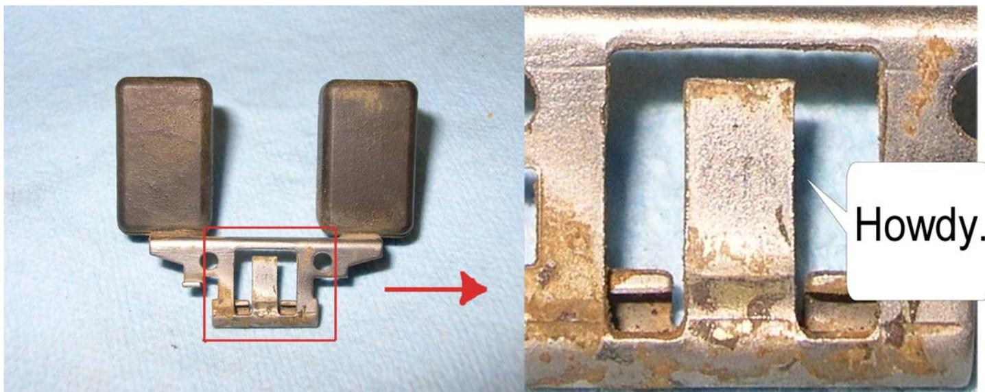
Yes and no. This reference to a "float level" (bad terminology, that – there is no such thing) can lead to confusion. We're not bending the float itself; that would be a Bad Thing™. We're bending a part of the float called a "tang arm".
