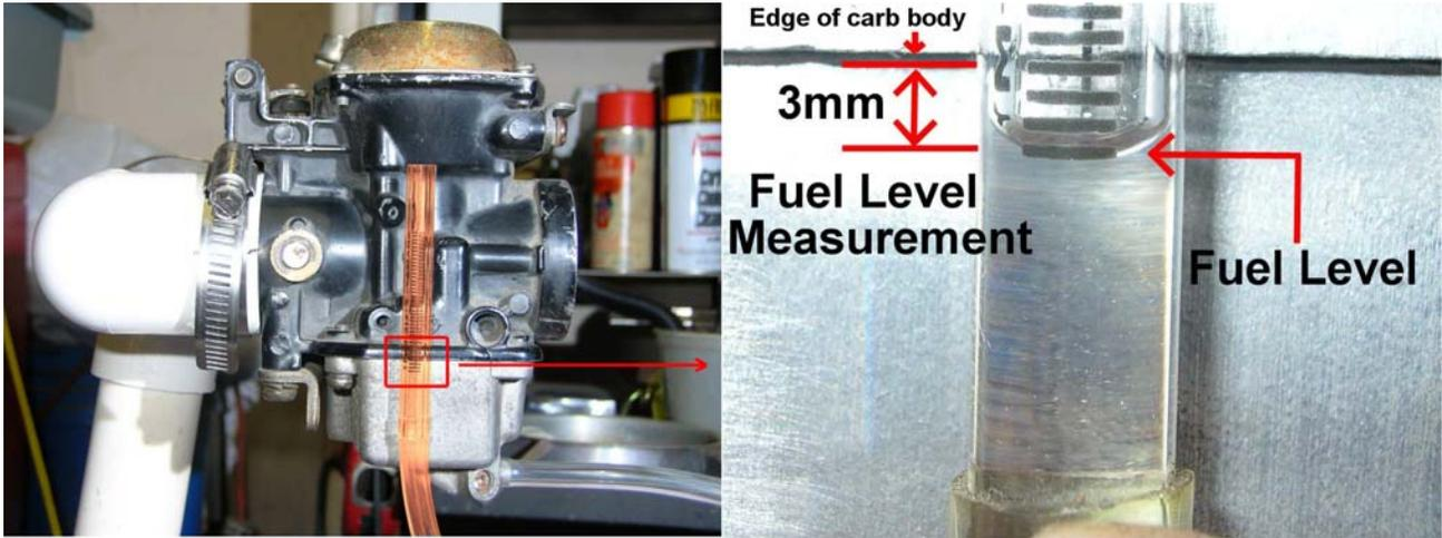
(If you're not using our [HCP1592](#) tube, but are using a plain tube without graduated markings on it, what you can also do is mark the float bowl to show where the fuel level should be before starting your measurements.)
