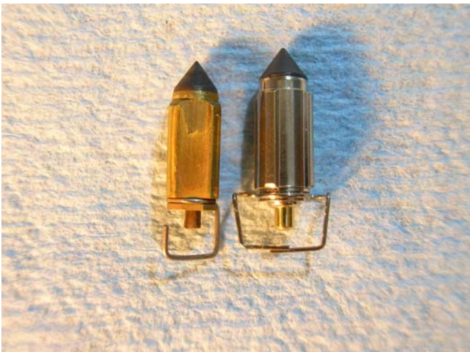
Replacement float needles – these should already be installed. Aftermarket parts, like the one on the right, can be 1mm longer than stock or OEM, seen on the left, so you want to be absolutely sure you use the same ones on all four carbs.
