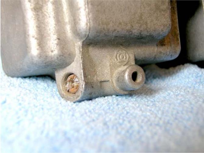
This picture shows why they might be needed. On this Hitachi float bowl (note the drain nipple on the right, below the logo), the head of the drain screw on the left is cammed out, and removing it will be difficult.
