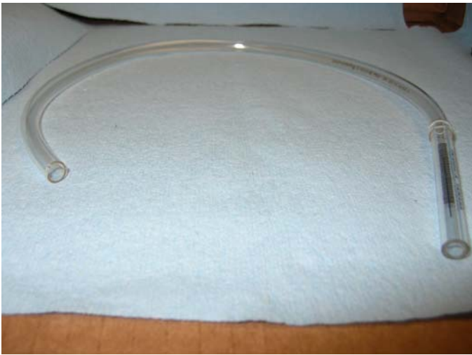
A clear tube with graduated markings (HCP1592) for measuring fuel levels.
