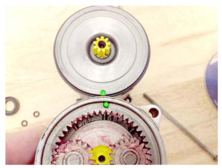
When installing the reduction gear assembly, take note of the alignment notch (green). Setting the armature gear into the reduction gears (yellow) takes a bit of patience to get everything lined up.
