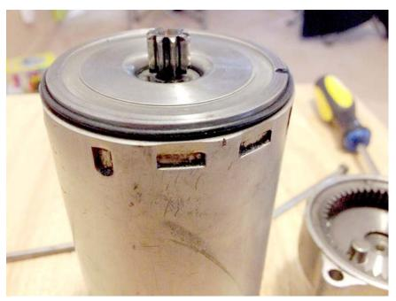
Install the outer o-ring for the reduction gear housing.
