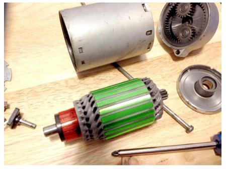
You want the armature (green) and comutator (red) areas to be clean. Use ONLY glass paper or metal polish on the commutator. You don't want to use anything harsher than this so as to not get particles embedded into the copper and cause premature wear of the new brushes.
