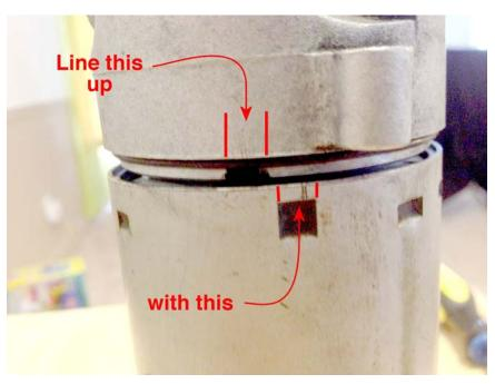
Align the notches (side view shown) as you press the entire assembly together. You can see here that the cap isn't (yet) aligned properly; when we suggested earlier that you make a mark on the housings, this is where that mark would come in real handy right about now.
