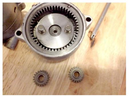
Now on to the reduction gear assembly. Pull out the reduction gears and thoroughly clean the inside and the gears themselves. I recommend nitrile gloves and lots of blue shop towels for this process.
