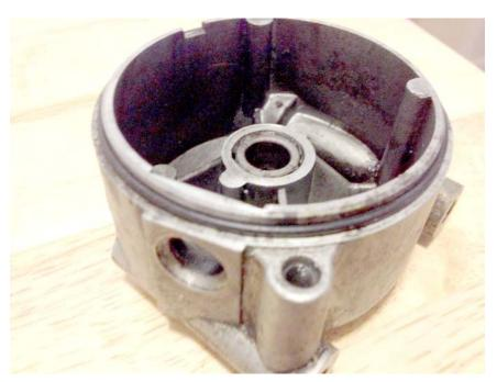
Then back to the brush end to install the other outer o-ring.
