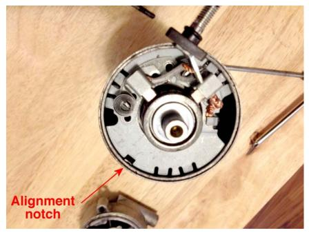
When installing the brush holder back into the stator housing, push the brushes into their holders and align the notch on the plate with the raised "peg" on the inside of the stator housing.
