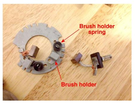
The new brushes need to be installed into the brush holder. If the brushes do not move freely you may need to sand the side or use a screwdriver to spread the holder out to accommodate the brush.
