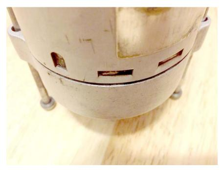
This picture shows the housings aligned properly, with the sides fitting flush. You will eventually get to this point...
