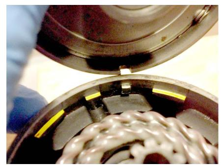
Close up view of the alignment notch. Note the yellow areas; these are what the end plate sits on. It does **not** sit flush with the outside of the housing.
