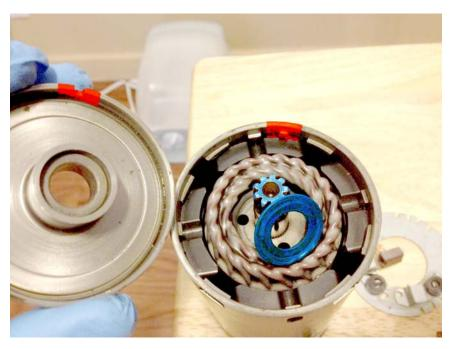
When installing the end plate before installing the reduction gear housing, note the alignment notch (neon red) and ensure to replace the washer (blue).
