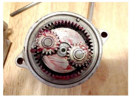
Once cleaned, grease the gears and re-install.
