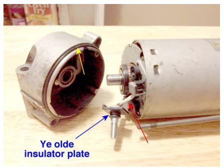
...so that you don't break the copper wires connecting the brush to the bolt (red arrow).
