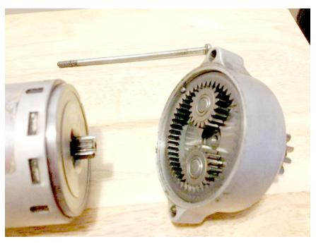
...and then you can remove the reduction gear housing from the stator housing.
