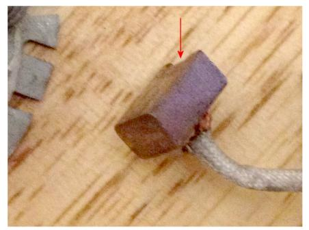
Note the red arrow pointing to the notch for the spring to set in. Make sure this is pointed away from the commutator when assembling.
