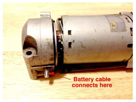
On the opposite end you need to pop off the brush plate cover but first, ESPECIALLY if you are only pulling it apart to check the brush length, you need to press the battery cable bolt through the housing...
