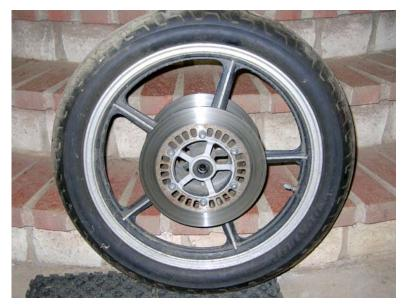
Here, we're going to go through the task of changing out wheel bearings. It's an infrequent task, to be sure, but a necessary one. Our example here is the front wheel from a California Maxim-X, 1985 vintage, and we'll start with the wheel already removed.
