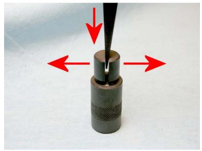
As you hammer on the drift rod, it expands the split on the driver. The plug grabs onto the inner race, and transfers the downward force of the drift rod onto the bearing.
