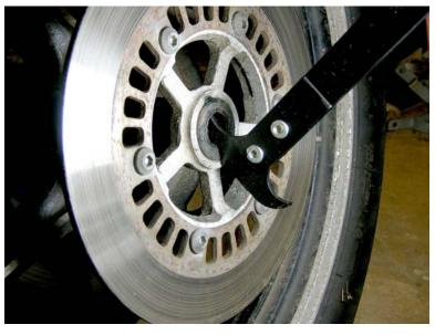
For removing said oil/dust seal, our HCP9801 seal puller tool comes in very handy here.
