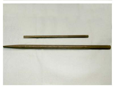
Also in the complete shop kit are two long drift rods; one end is tapered. The tapered end fits into the slot on the driver.
