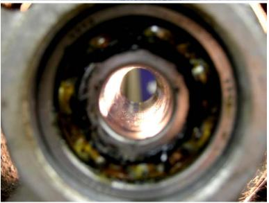
Ordinarily, one would just grab a hammer and a punch or similar tool, stick the punch through the hole on one side, and start driving out the bearing on the opposite side by tapping on the inner race. That might not work here, because there's a spacer between the two bearings – meaning it's difficult at best (if not flat-out impossible) to rest your punch on the inner race. A Royale-With-Cheese-pain-in-the-posterior, if you will.
