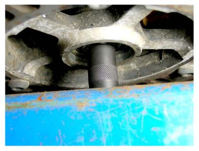
Since the split collar won't want to grab at first, you might want to have a helper hold it in place while you start tapping, or stand the wheel up on the end of the collar while you give the drift rod a few good whacks to get it started. Then put the wheel back up on its rubber and keep pounding.
