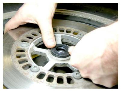
Lastly, the new seal. A light coat of silicone grease around the inside and outside, and you should be able to press it into place. Lightly tap around the outside with a punch (or the old bearing again) if necessary.
