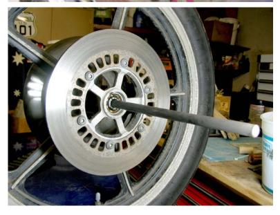
Take the drift rod, insert it from the other side, and fit the tapered end into the slot. Now you can use a hammer, or perhaps better, a small 2 or 3 pound hand sledgehammer.
