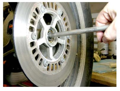
What you can try is to shift the spacer over far enough to open up a spot to put the punch on. A long screwdriver or perhaps a long ratchet extension would be called for here.
