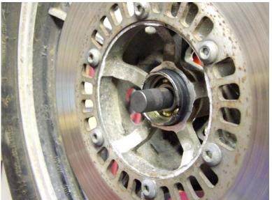
To use the tool, take the appropriate-sized driver, and put the slot end into the bearing hole. The rest of the plug should rest on top of the inner race.
