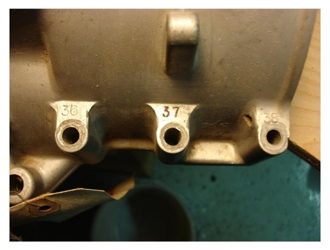
All over the upper and lower crankcase sections, you will find small cast numbers that range from 1-39 (actually, different number ranges on different engine styles; we're using the 650 - 900cc engines for this example). These numbers are always just beside a drilled passage hole in the case, and these bolt holes are all for the fasteners (bolts) that secure the upper crankcase section to the lower section.
