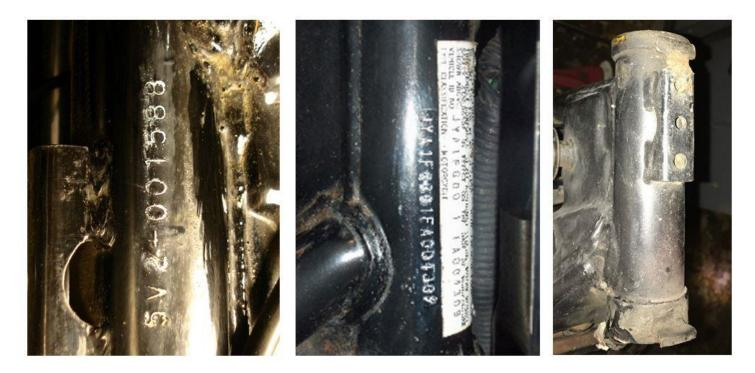
On the **right** side of the steering bearing headpipe, there will be either a "short" version of the full VIN (or, on later model bikes, the full 17-position VIN) that is physically **stamped** into the metal (we've filled in the letters/numbers in the images above with white paint to make them look more visible).
