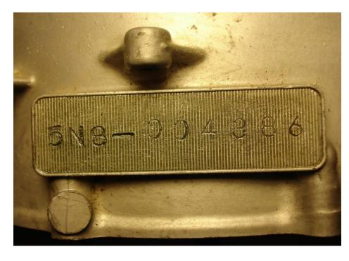
On the upper engine case, just behind or just beside the clutch cover on the right side of the engine, you will find a small, flat "ribbed" (to prevent re-stamping) machined pad that faces up (towards the sky).
