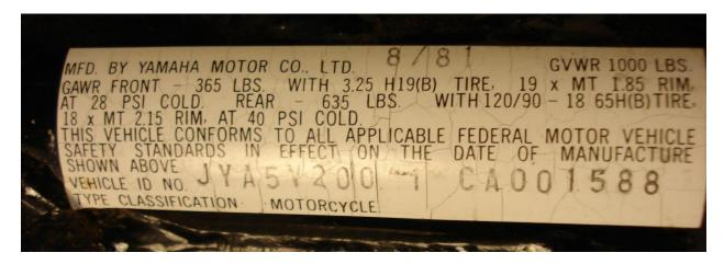
This vinyl sticker will be found on the left side (or, on some models, directly in the center, facing almost straight forward) of the steering bearing "headpipe" or "frame vertical tube" behind your headlight housing. This decal measures about 1-1/2" x 4" and is located vertically on the headpipe (in other words, you have to rotate your head 90-degrees to read it). So in the above image the left side of the image would be "up" or at the <u>top</u> of the headpipe.
