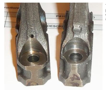
The oil spray passage hole allows pressurized oil to be sprayed onto the cylinder walls, aiding lubrication of that area.
