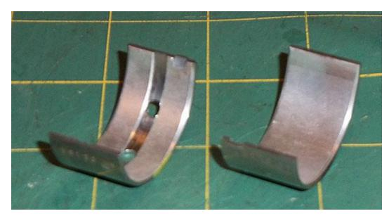
2) there are two different types of crankshaft main journal bearings: those *with* and <u>*without*</u> oil passage holes:
