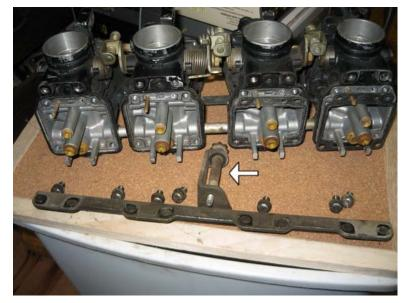
Bottom bracket removed. Note the idle adjusting screw.
