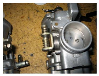
Stick the stud and spring back in the hole and put some tension on it
