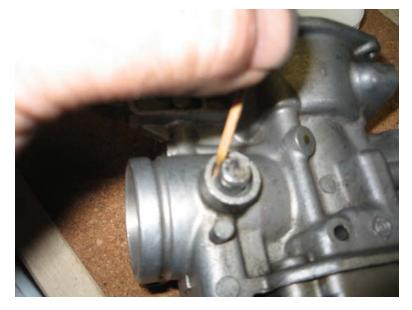
Insert the shaft, then add a thin film of silicone grease to the shaft
