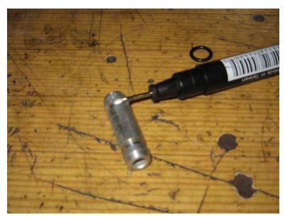
A light coat of silicone grease in the groove that the o-ring goes into
