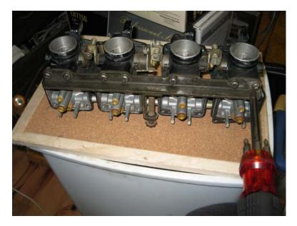
Remove the mounting screws from the bottom bracket
