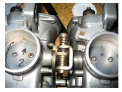
Slide the tab from the neighboring throttle shaft between the adjusting screw and the stud
