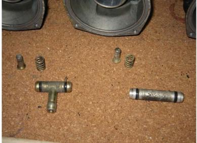
Closeup of the fuel rail tubes. Remember: the long one goes between 2 and 3.
