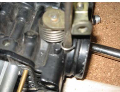
Unhook the spring from the throttle shaft
