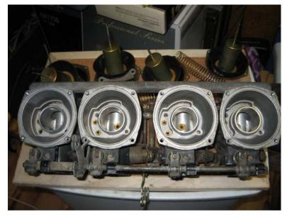
The springs and diaphragm/pistons are out
