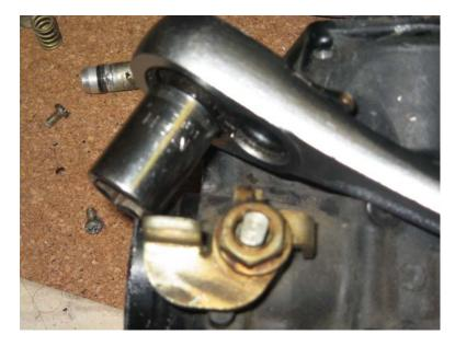
For the inner two bodies, the nut holding the shaft in wants a 12mm wrench/socket
