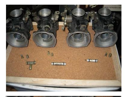
The fuel rail tubes (with o-rings) and the little studs/springs from the bottom part of the sync screws. Don't lose them!
