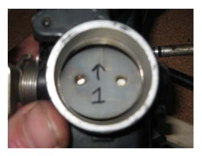
Remove the two screws holding the butterfly to the shaft
