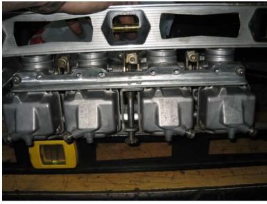
Use something (a block of wood or another level) to gently press down on the other side of the carb bodies and start adding screws from the outside in (and there's that Loctite thing again)
