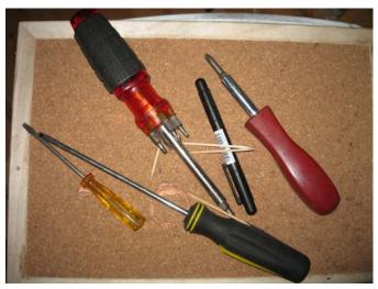
A set of good-fitting screwdrivers. Stripping the screw heads is a Bad Thing<sup>tm</sup>.
