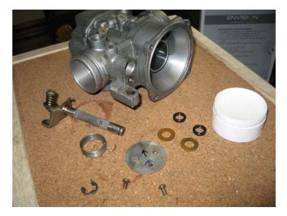
All the bits ready to go back in. Note the little tub of silicone grease.
