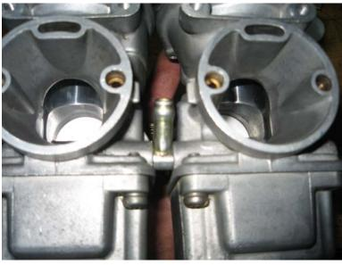
Press the other side of the fuel rail tube into the other hole
