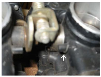
Here we see how the throttle shaft spring hooks onto a little stud.
