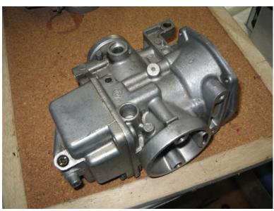
Switching back to my (somewhat cleaned up) working set now. Note that I've reinstalled the float bowl; it's been suggested to keep it bolted on to protect the float pillars from damage.
