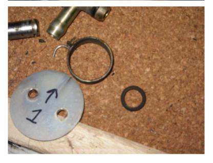
The butterfly, throttle shaft spring, and outer seal
